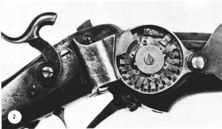
2nd model Sharps priming mechanism
