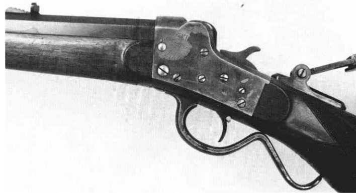
"Medicus Skinner" no. 12. "Medicus" was the nom de plume of Dr. S. A. Skinner, friend and researcher of Dr. Mann, author of "The Bullet's Flight". Has operational lever as shown on patent drawing, but regular Hepburn action. Cal. 32-40 breech & muzzle loading.
