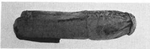
The first American revolver cartridges were very similar in construction to those of the percussion pistols, except that they had conical bullets. Here is the rare yellow paper cartridge for the Colt Dragoon revolver, circa 1856, with 232 grain bullet and 30 grains black powder. The latter is a considerable reduction from the 50 grain charge for the Walker, and the 40 grain dragoon charge of 1850.
