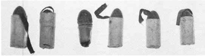
On the left are three 38 bore (.50 calibre) cartridges, the open specimen with a glued-on skin case; the others are 54 bore.
