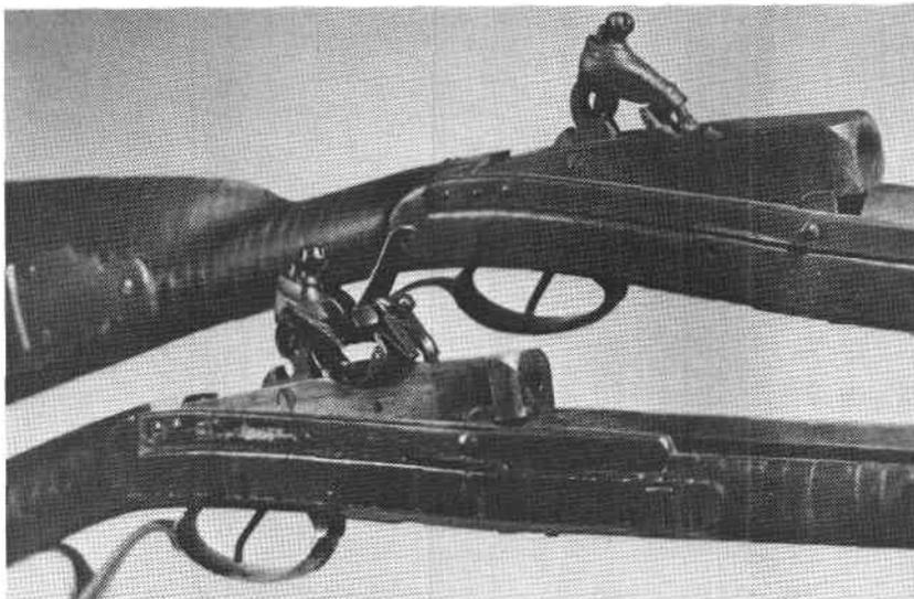
Fig. 9. Two post-1815 Hall breechloaders, one converted to percussion.
