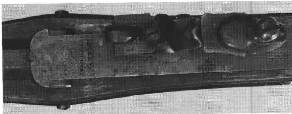
Fig. 11. Post-1815 Hall breechblock showing typical Hall markings.
