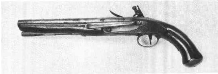
Reverse of the 1812 U.S. Navy J. Henry pistol showing the attachment of the belt hook by the rear lock plate screw.
