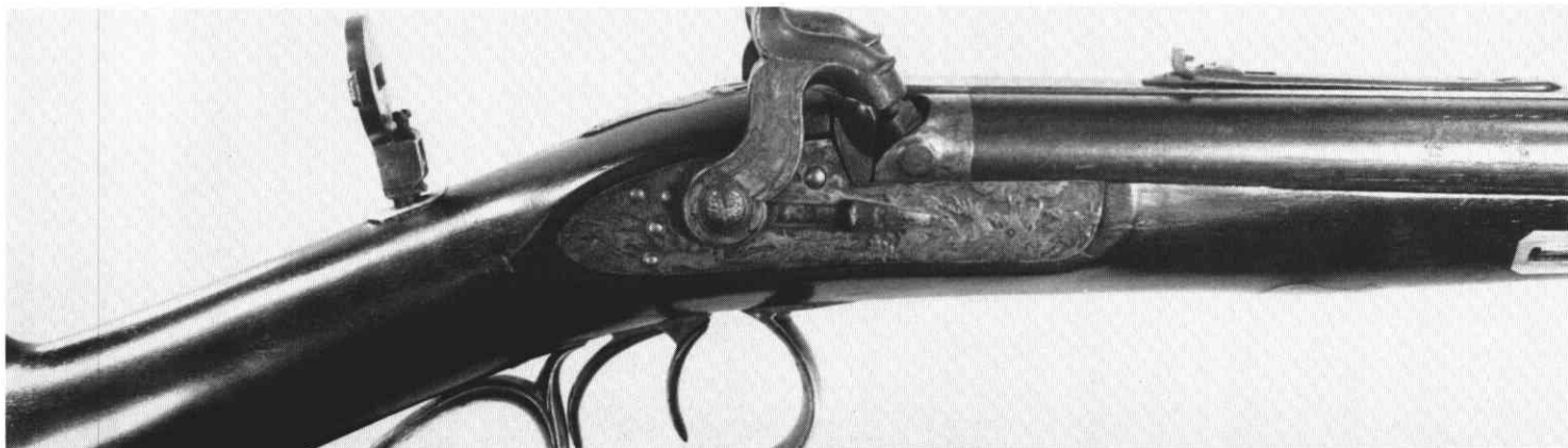
The lock, peep sight, and trigger guard of the Rogers rifle . . .
