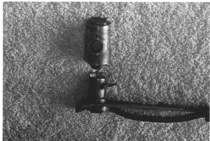
The swivel breech and its lever.
