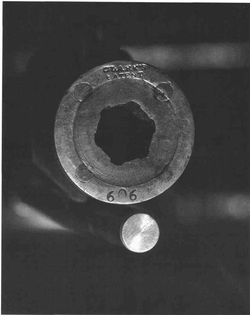
Figure 6. Detail of false muzzle stamped “Clark’s/Patent/606.” Heads of the four alignment pins are clearly visible, having passed entirely through the length of false muzzle. Photo courtesy of Ron Gable.
