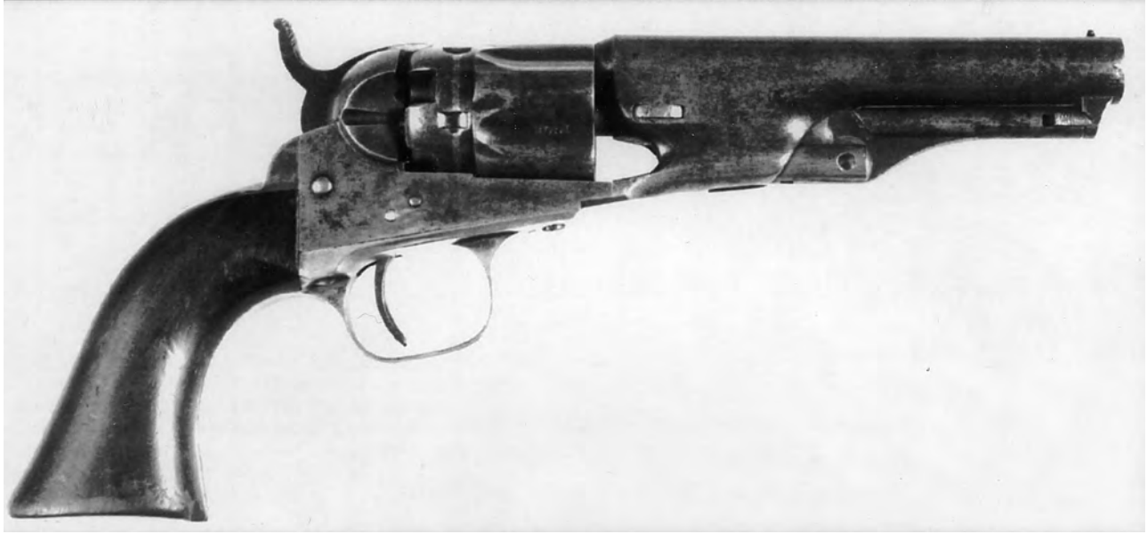
Figure 1. "1862 Police" .36 caliber percussion pistol. Note round barrel, "creeping" ramrod, and fluted cylinder. Frame, grips, back strap, triggerguard and other parts are common with the "Pocket Model of Navy Caliber" in Figure 2. Robert B. Berryman photograph.
