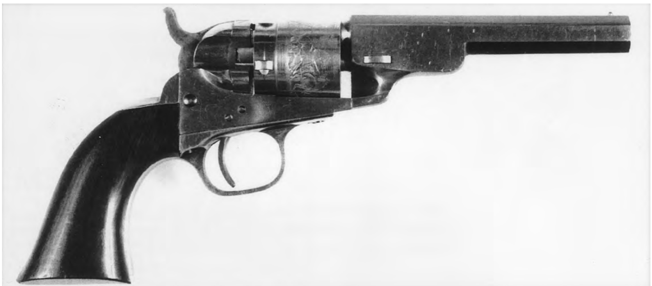
Figure 4. New Model Breech Loading Pocket Pistol. Without loading gate, converted from a previously finished "Pocket Model of Navy Caliber.". Robert B. Berryman photograph.
