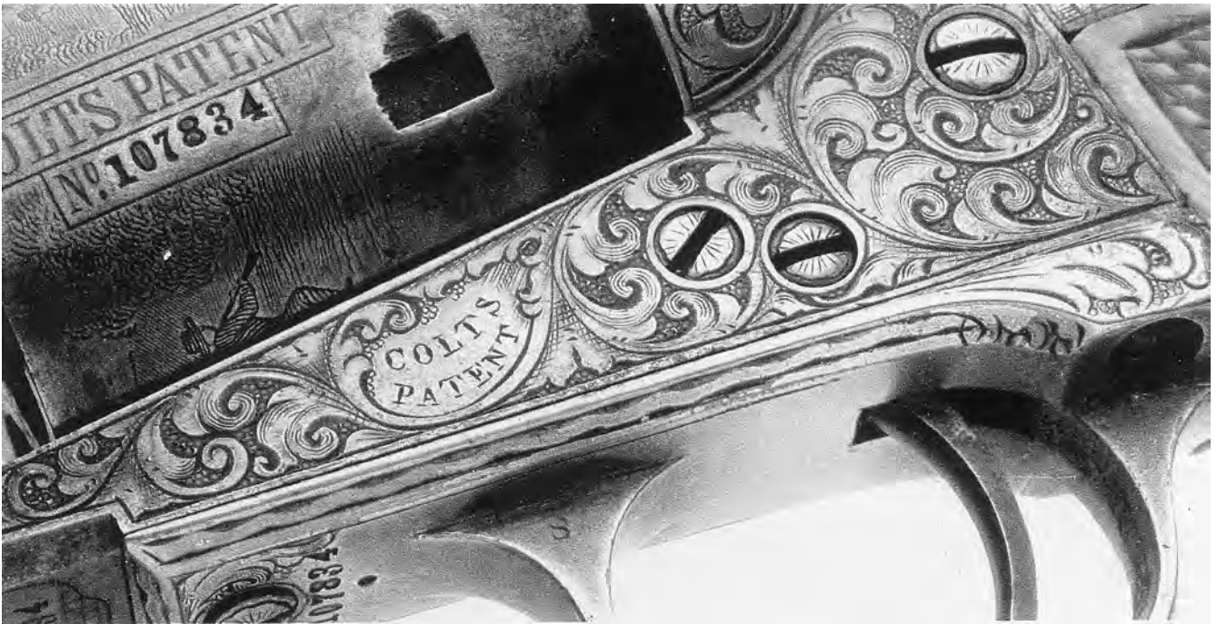
Figure 5. Gustave Young engraving on the frame of an Old Model Pocket Pistol. Note stippled background. Darrow M. Watt Photograph, Courtesy of Mr. Watt and Robert M. Jordan.
