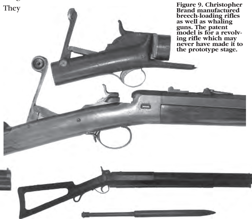
Figure 10. Christopher Brand's classic whaling harpoon gun. These were made in three bore sizes and fired the explosive harpoon shown in the photo.
