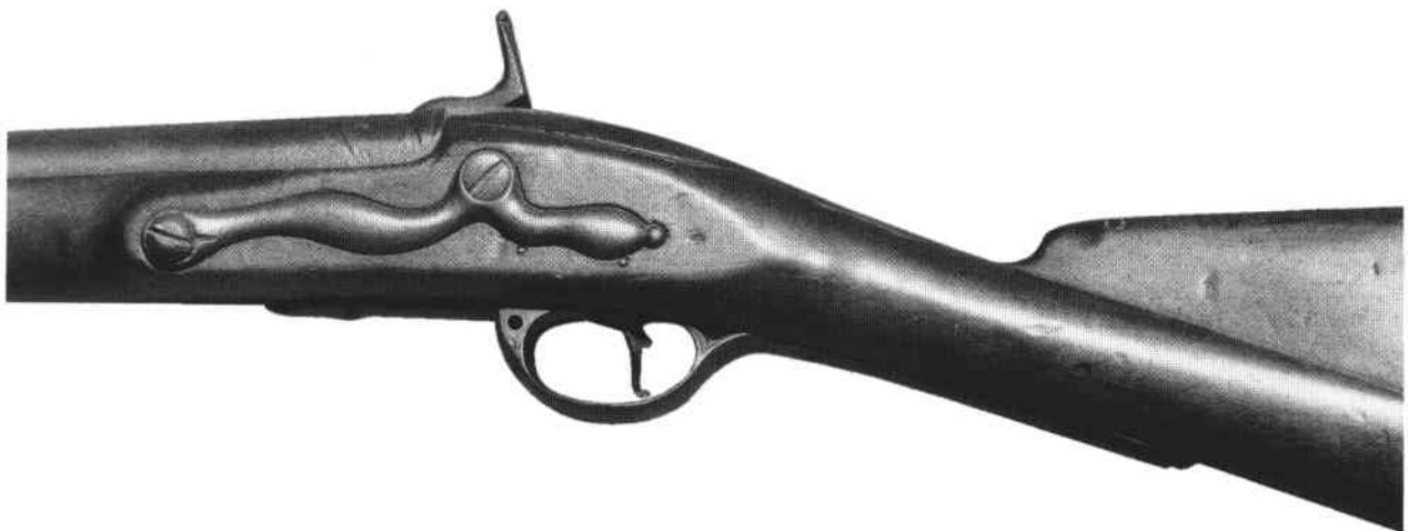
Figures 6-9. British Long Land Pattern musket converted to civilian use as a shotgun, circa 1840. One of the rarest examples of an American War period firearm. Most have been reconverted to flintlock percussion in an attempt to recapture a perceived original form.
