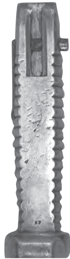
Figure 24. Model 1855 sword bayonet guide slot.
