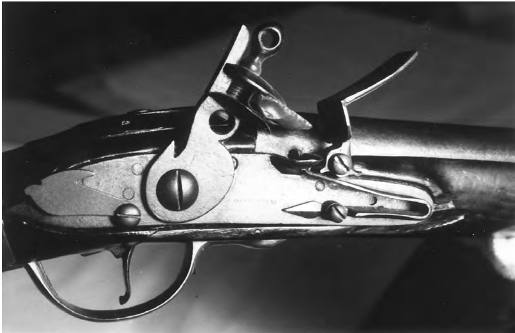
Figure 19. A Dog-lock muskets of the pattern discontinued by the Board of Ordnance after 1715 remained a popular design for export arms into at least the 1740s. All the tools and jiggers existed, and they were cheap and strong. Courtesy The Valley Forge Historical Society.
