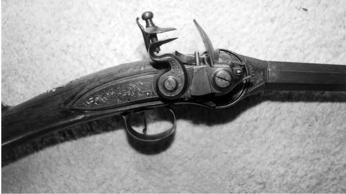
Figure 16. A Lorenzoni-system breech-loading repeating rifle by William Wilson (I) ca. 1770. Private Collection.
