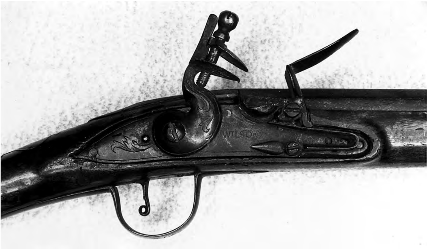
Figure 5. A typical Wilson trade gun lock used on the lowest grades of fuzees for the North American Indians for most of the 18 th Century. The single border line on plate and cock body, the very simply engraved foliate scrolls and the name in plain block letters, are, along with the “plain” lock mechanism (lacking either tumbler- or pan-bridle) and the straight “pillar” comb of the cock, characteristic of this grade of lock. This example still has three screws attaching it to the stock through its dragon sideplate. There are a great many structural variations found on Wilson trade-gun locks all within a broad general category. Private Collection.
