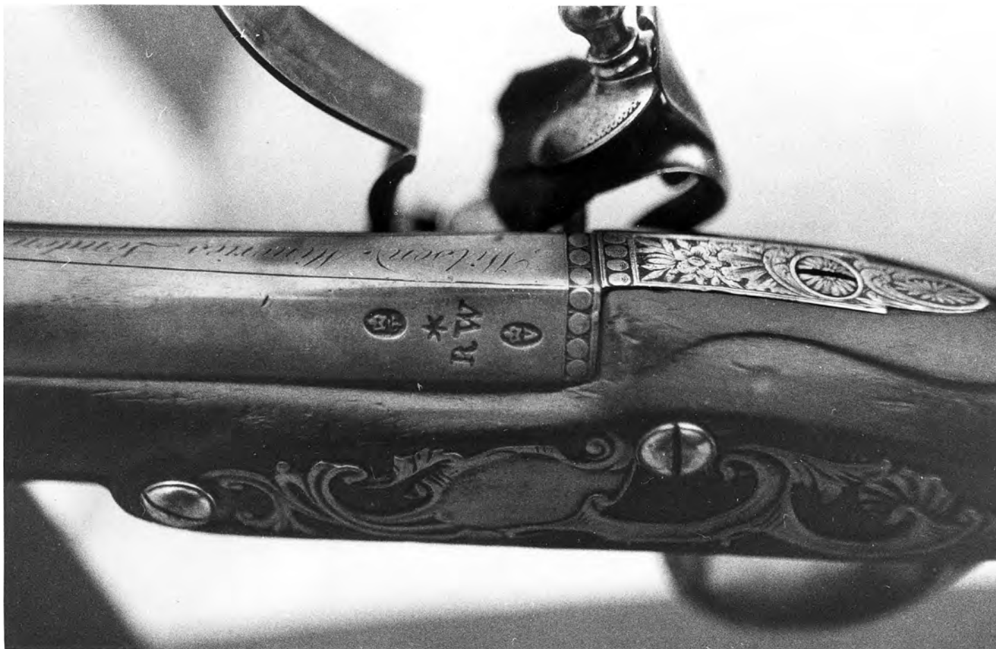
Figure 12. Breech markings on a pistol by William (I) Wilson. Note the full address engraved on the tapering flat of the brass barrel. It is probably significant that most of these full addresses are found on brass barrels which were softer and therefore cheaper to engrave. Private Collection.
