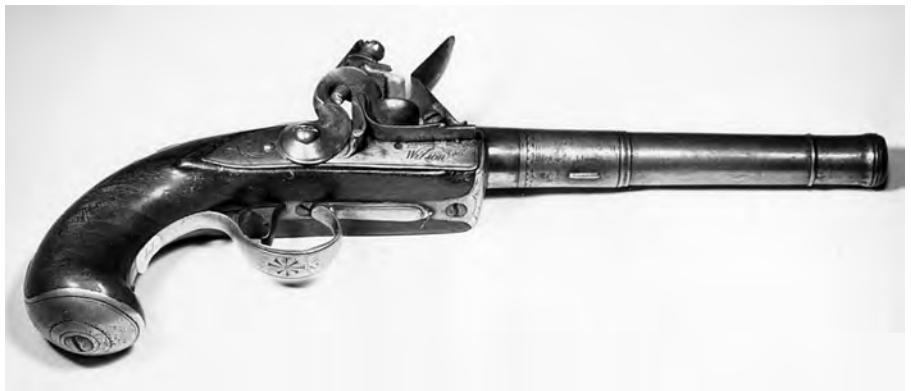
Figure 1. A rifled breech-loading pistol by Richard Wilson in an uncommon style which enjoyed but a brief popularity in the 1740s. Despite the advanced technology, note the absence of a pan-bridle. Private Collection.
