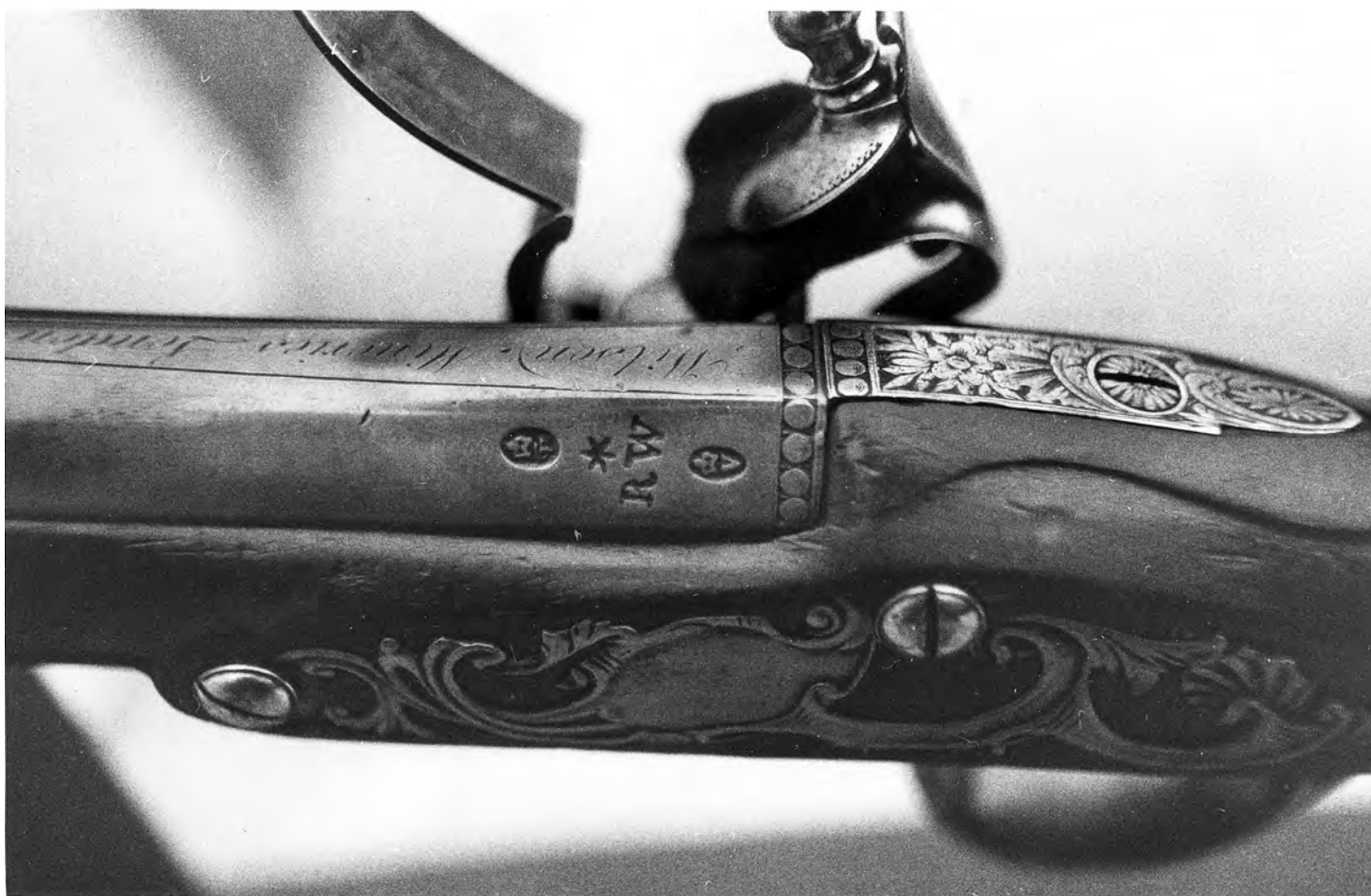
Figure 12. Breech markings on a pistol by William (I) Wilson. Note the full address engraved on the tapering flat of the brass barrel. It is probably significant that most of these full addresses are found on brass barrels which were softer and therefore cheaper to engrave. Private Collection.
