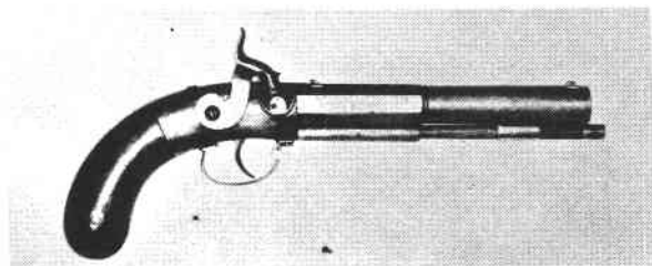
#11 H.E.DIMICK & CO., ST.LOUIS, 2 LINE, AMERICAN MADE HALF ROUND HALF OCT. 6" BBL., .44 CAL, ALL INSPECTOR MARK INITIALS CHECK WITH KNOWN DIMICK EMPLOYEES, MARKINGS ON BBL DIE STRUCK, TYPICAL ST.LOUIS PATTERN
