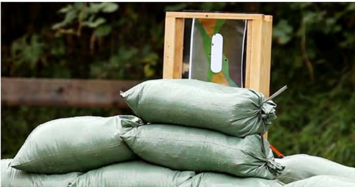
Figure 16 b. The target trap used in our trial containing a simulated backlit loophole aperture. (Holly Marcus)
