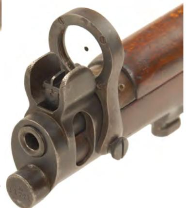
Figure 9. b. The Martin sight's objective fixed to the muzzle cap of an SMLE. Note the prominent 4 MOA dot aiming point. (Author)
