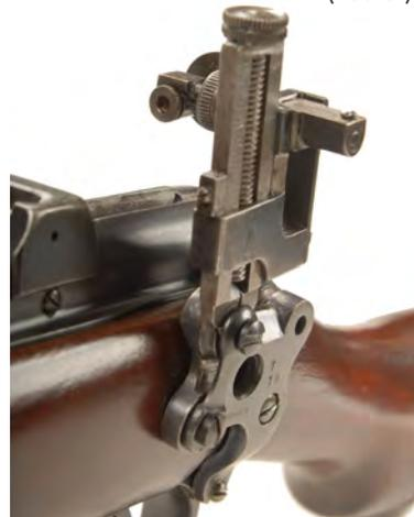
Figure 9.a. The ubiquitous No.9 micrometer adjustable target rear sight. Note the tiny ocular lens for the Martin sight inserted at the front of the windage arm. The No.9 rear sight was used for both the Martin and B.S.A. Galilean optical sights. (Author)
