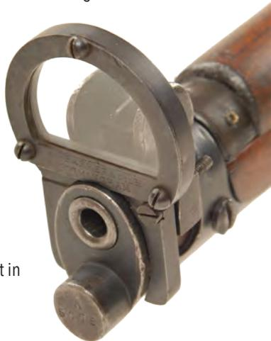
Figure 7. c. Close-up of the Lattey's objective. Note the clamping arrangement engaging the lightening cut in the muzzle cap. (Author)
