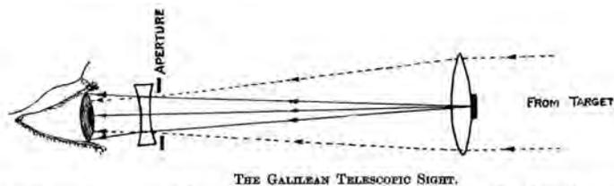
The continuous lines represent the rays from the aiming mark, the dotted lines those from the target.
