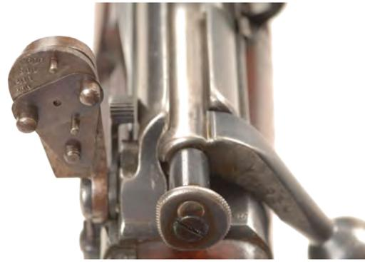
Figure 8.a. The Ulster/Neill rear sight, fitted to the dumbbell spring at the rear of the receiver. It is graduated from 200-600 yards; the earlier variants were only marked to 200 yards. (Author)
