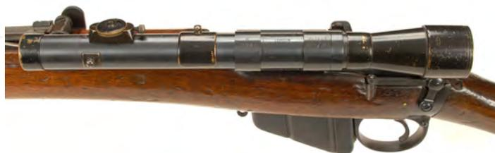
Figure 6 - Receiver area of an SMLE Mk.III fitted with a Periscopic Prism Co. telescopic sight. The magnification of this sight was the same as that of the Galilean sights, and both were in service in 1915. (Author)
