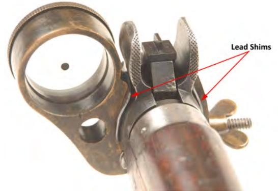
Figure 8. b. The offset Ulster/Neill objective with its prominent 4 MOA dot, a vestige from Bull's Eye shooting. Note the lead shims that were employed (today as in WWI) to stabilize the clamping of the sight in the muzzle cap's lightening grooves. (Author)
