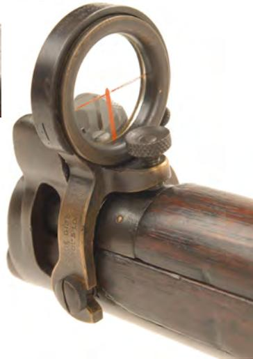
Figure 10.b. The objective of the Gibbs sight, with probably the most precise aiming point. (Author)
