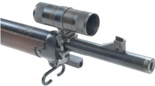
Figure 11. The B.S.A. sight was patented in 1912 and thus was already in use on target ranges before WWI. It also used a No.9 micrometer rear sight. (Author)
