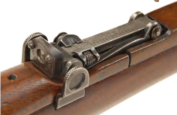
Figure 7. b. Close-up of the Lattey's ocular lens holder attached to the standing leaf of an SMLE Mk.III. The radius of the handguard behind the sight needed to be relieved slightly to allow full depression of the elevator, otherwise its graduations are useless. (Author)
