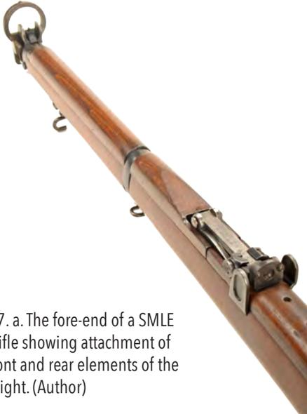
Figure 7. a. The fore-end of a SMLE Mk.III rifle showing attachment of both front and rear elements of the Lattey sight. (Author)
