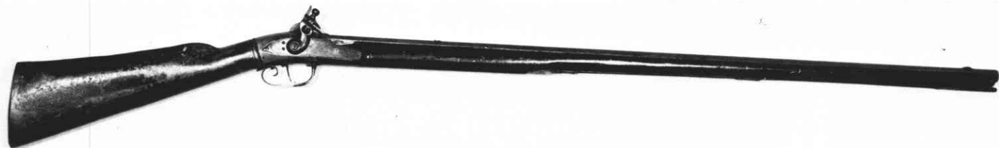
Fig. 3: The Isaiah Lukens air rifle originally indicated by Charter Harrison as the "Lewis & Clark gun". Overhead striker in conjunction with flint hammer, butt shaped (not flask) reservoir.
