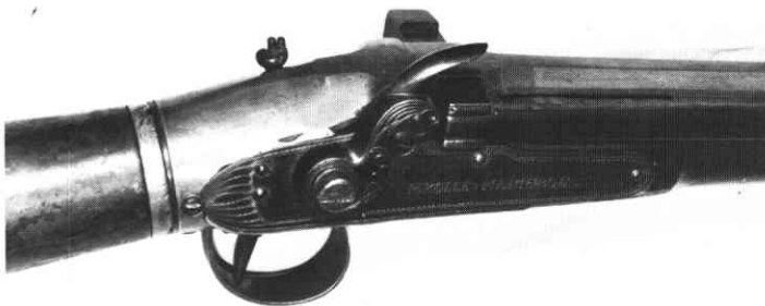
Fig. 2: M. Kollé of Marieboe — The Girardoni magazine on a brass, smooth bore, flask butt, pneumatic.
