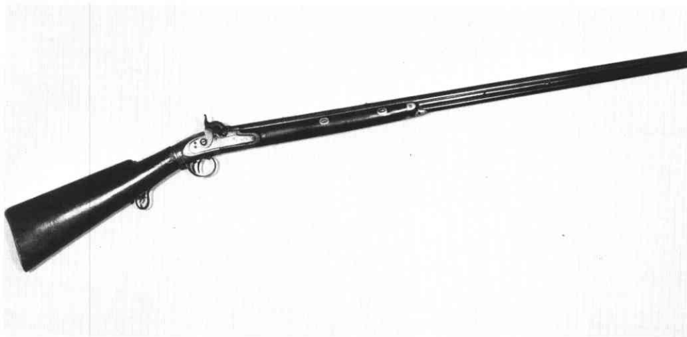
Fig. 6A: J. KUNZ, Philadelphia, of the 1830 period, gold bands, silver inlays, engraving, and two barrel system: upper percussion, lower pneumatic. Cased with accessories.
