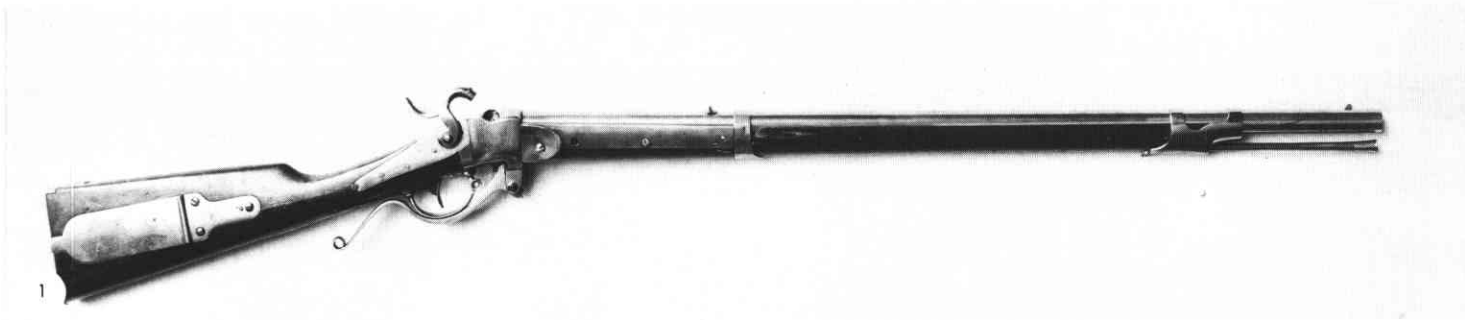
Sharp's patent model, built on M1842 Mississippi rifle.
