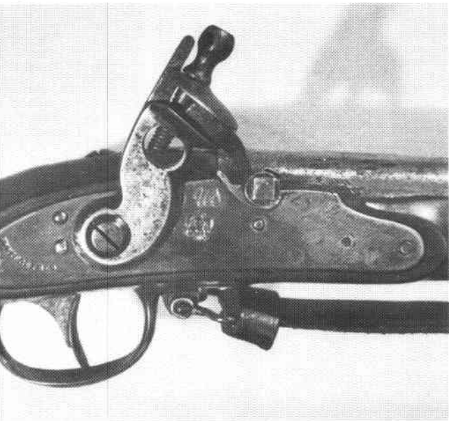
Figure 1 Flint hammer striker conversion of an 1808 Musket
