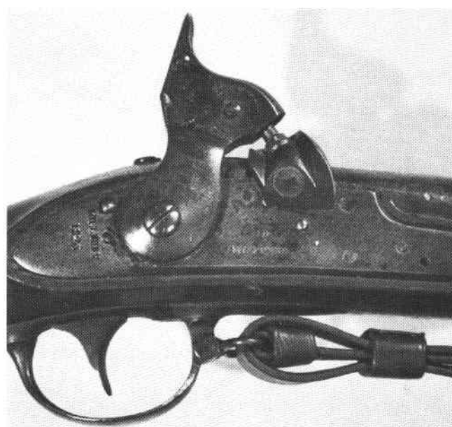
Figure 9 Ward Primer alteration of an 1816 musket
