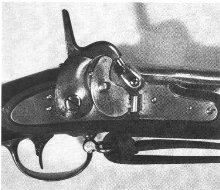
Figure 8 Remington Maynard conversion (second type) of an 1816 musket.
