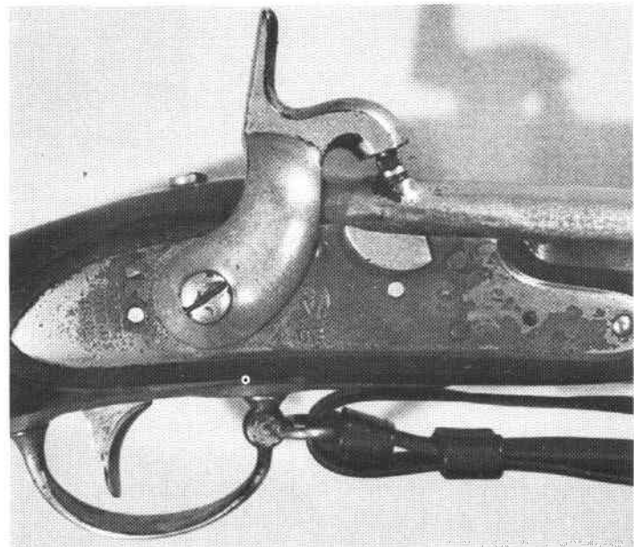
Figure 4 Cone alteration of an 1816 musket
