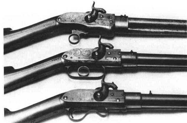
Jennings Rifles. Upper: A repeater; Center: a single shot, and, Lower: converted to muzzle loader.
