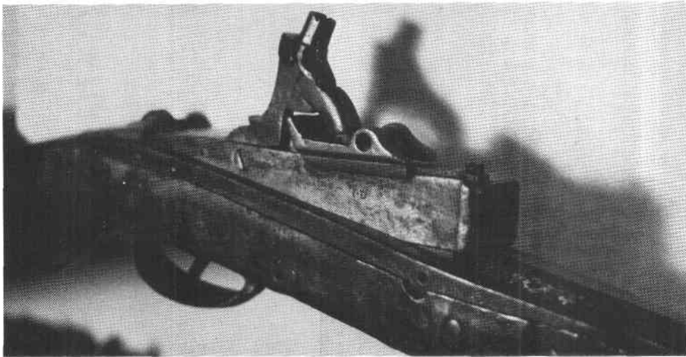
Fig. 6. An early Hall breechloader with breech open, converted to percussion and frizzen removed (circa 1812).
