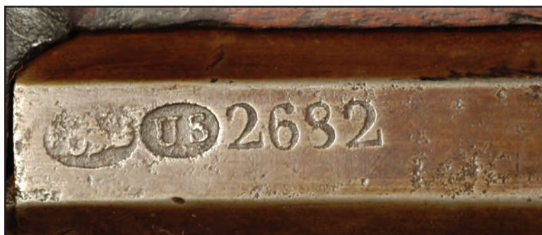
Shows horizontal lines on serial numbers. These lines are also on #2682 and presumably on all 4015 model 1803 rifles.
