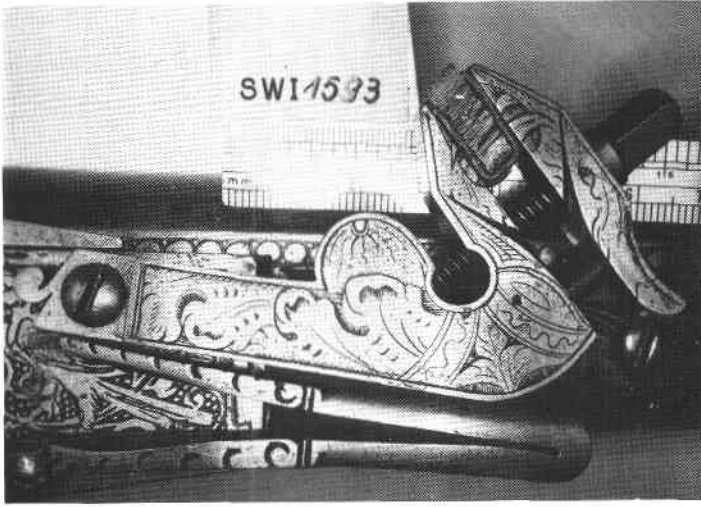
The replaced cock on the pistol. It should be noted that we do not undertake the reconversion of former flint locks. This is a matter of principal.
