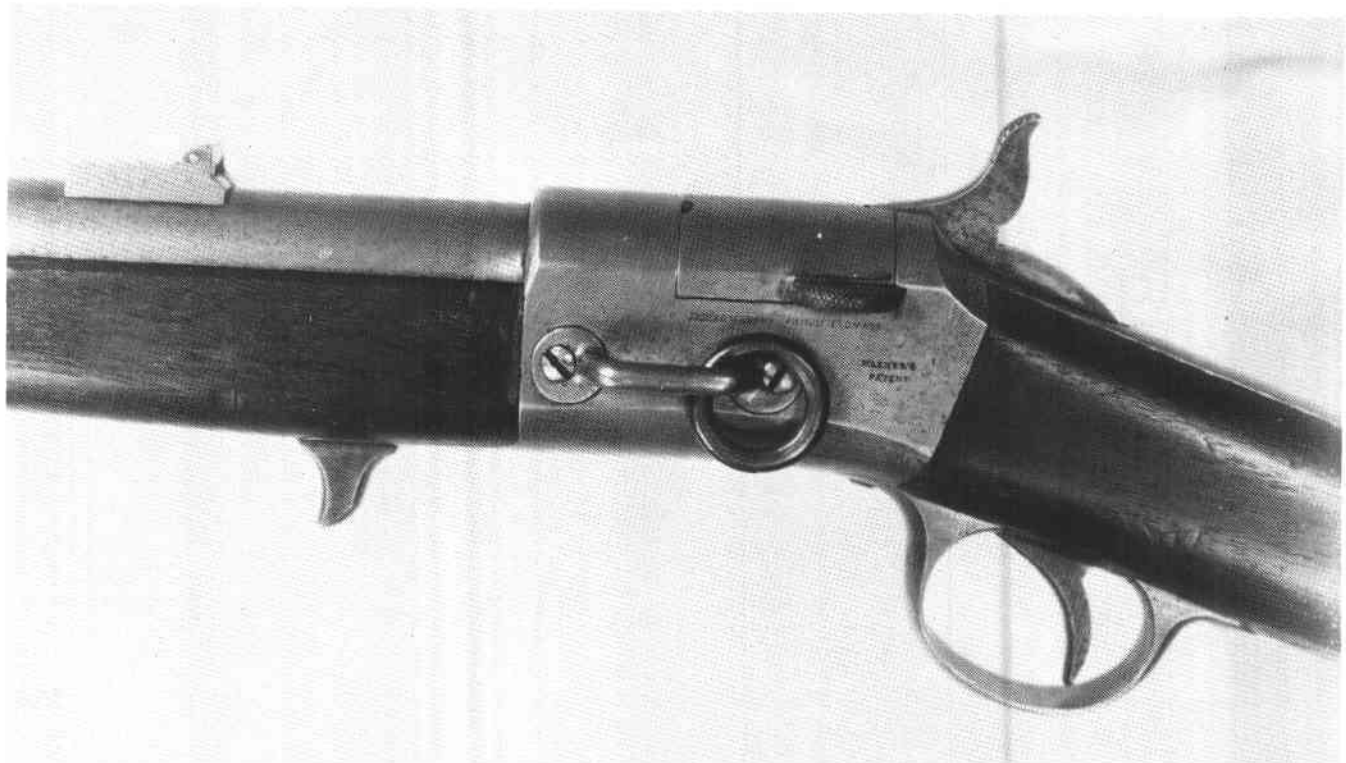
WARNER IRON FRAME Breechloading Cartridge Carbine (United States Government Trials of 1865 Carbine). .50 caliber (.56-50 Spencer). Finished bright overall. No serial number. Marked on left side of frame: "JAMES WARNER, SPRINGFIELD, MASS., WARNER'S PATENT" The breechblock is released by pressing forward on a flat (11/16" long) button, which is knurled along the curved periphery. Breechblock swings up and over to right side in usual fashion. Rear sight is graduated for 300, 500 & 800 yards. The 20 inch barrel has 3 wide lands and grooves, with clockwise twist. Overall length is 37-1/8 inches. Sling ring bar on left side of frame is one inch long (center to center of the bar itself. Stocks of walnut. Weight is 6-1/4 lbs. (Andrew F. Lustyik Collection)
