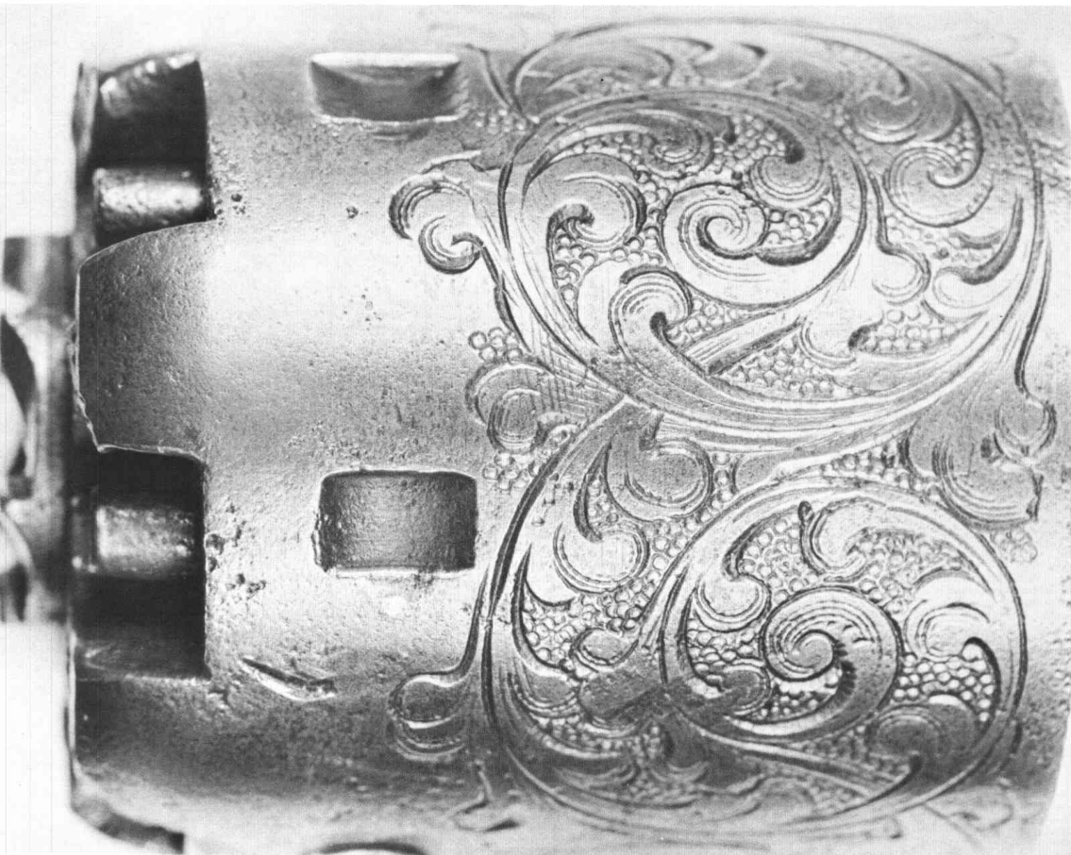
Figure 3. This is a portion of the Colt cylinder showing lines of the original rolled scene under later scroll engraving, the result of the faker's failure to remove all of the original scene for fear of reducing the diameter of the cylinder too far.
