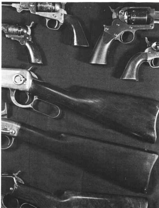
Figure 7. This photo shows a Colt 1851 Navy, a Paterson Colt and a Colt .36 Pocket Pistol all with shellac finishes or a heavy shellac undercoat; also a single action Starr with an oil finish, a 94 Winchester carbine with varnish finish, a Smith civil war carbine with oil finish and a deluxe .92 Winchester with shellac finish or a shellac undercoat.
