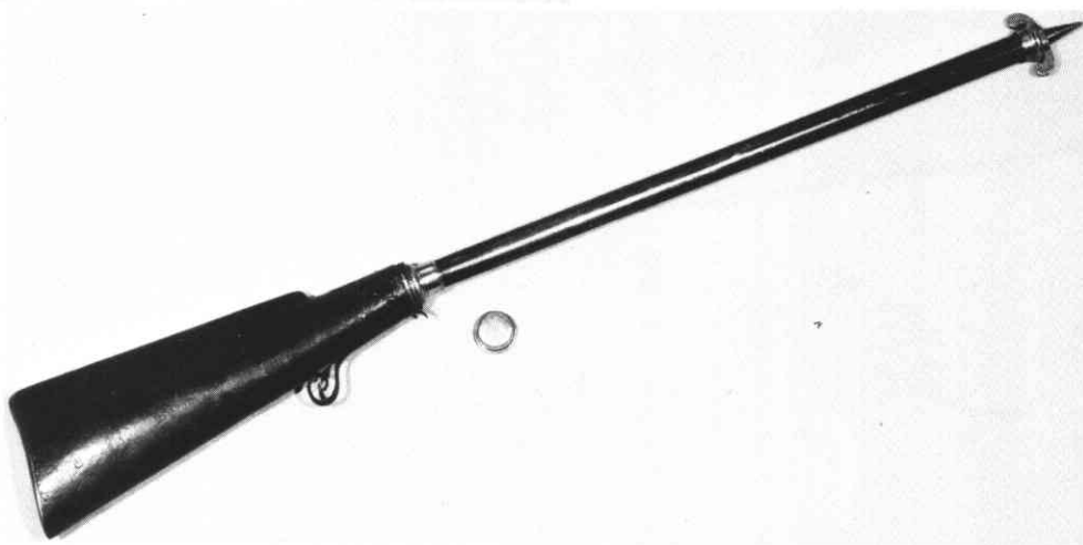
Fig. 7: Philadelphia butt reservoir attached to its pump ready to be screwed into shoulder-level point on tree for pump-up.
