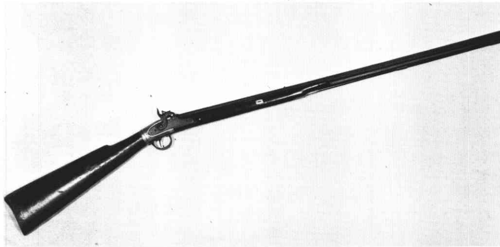
Fig. 6: J. KUNZ, Philadelphia, showing improved skills of about 1830 — gold bands, top flight engraving, etc. Forty shot butt reservoir half-stock model.
