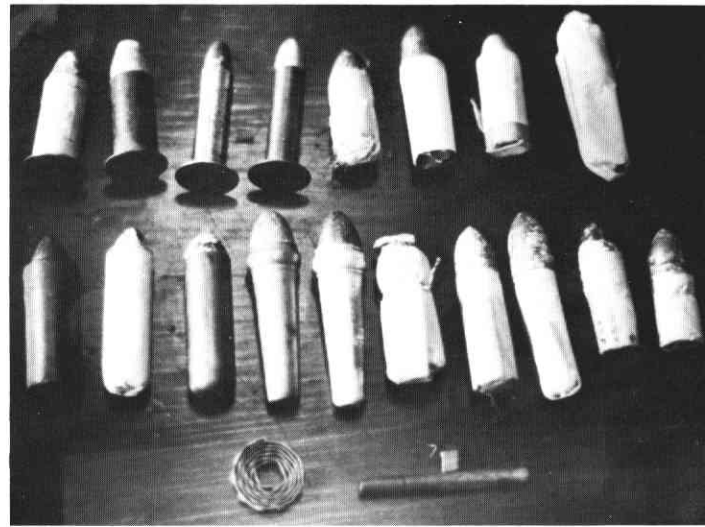
Assorted carbine cartridges (and a Whitworth bullet) with Maynard tape and Sharps disc primers.
