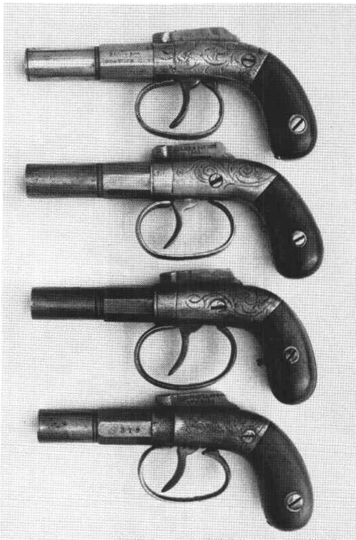
Bacon & Co. small frame bar hammers with Allen & Wheelock, Blunt & Sims, and Manhattan copies.
