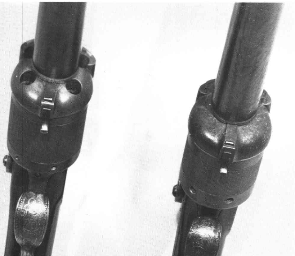
A comparison of the cylinder fore end cap on the 1st model guns. With the exception of the rifle on the left, all James Millar patent cylinder guns have a solid fore end cylinder cap. The gun on the left has four ports of the proper caliber which could be gas ports or could be used to facilitate loading of the cylinder.
