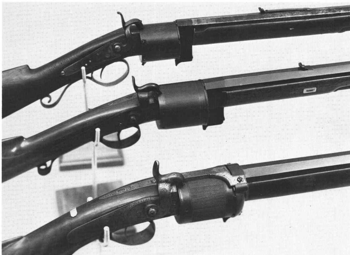
The three basic types of Miller guns: the bottom gun represents the James Millar patent and is type 1. The middle gun is the type 2 model with the pill-lock ignition system but lacking the features of James Millar's patent. The top gun is type 3 and is similar to type 2 except that it uses percussion caps.
