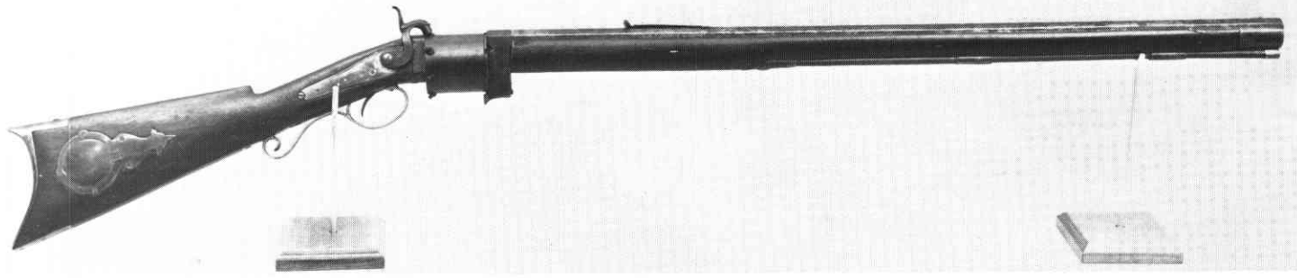
One of the few fullstock Miller revolving cylinder rifles. This gun is marked "J. & J. Miller Rochester" and has the percussion cap ignition system. Author's collection
