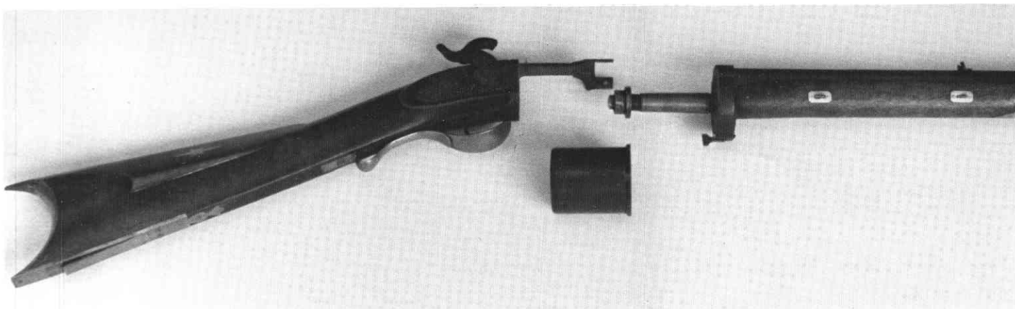
James Millar's personal gun disassembled to illustrate the bridge or top strap over the cylinder and also the cylinder fore end cap, two of the main features of his patent. Richard Harvey Millar
