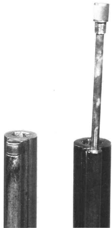
A comparison of the unusual rammer or cleaning rod found on at least three of the 1st model guns. To extend the rammer, the fore end was unscrewed, pulled out and further unscrewed to secure it in the extended position.
