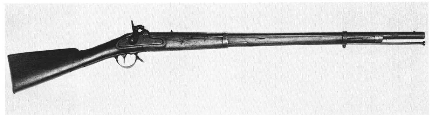
Another Florence Armory rework. A 33 5/16" barrel with Lamb characteristics, now .63 caliber smoothbore. Other parts may be from MJ&G, Clapp, Gates & Co., and Searcy & Moore.
