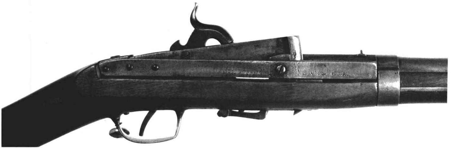
The elbow lever pushed upward and the breechblock ready for loading.
