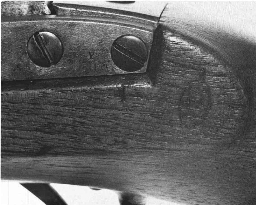
The acceptance mark of Nahum W. Patch, government inspector at North's army. The small "P" between the chock screws is Patch's sub-assembly mark.
