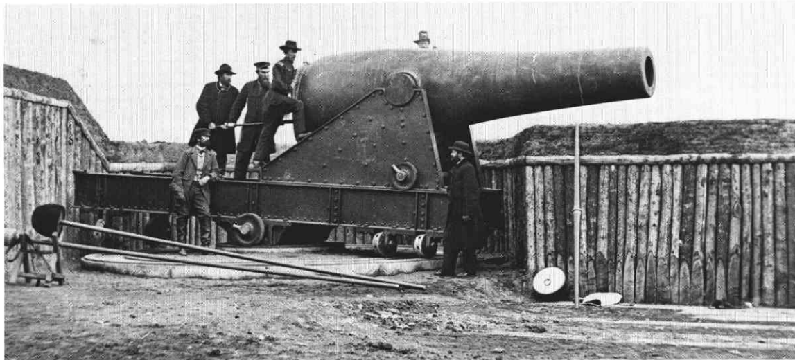
Army 15-inch Rodman gun at Battery Rodgers, Alexandria, Virginia. Assistant Secretary of the Navy Fox ordered Dahlgren to design a navy 15-inch gun when he saw a piece similar to this after the Battle of Hampton Roads. Dahlgren claimed that Rodman used the lines of his 11-inch gun to design the army 15-incher. National Archives photo.
