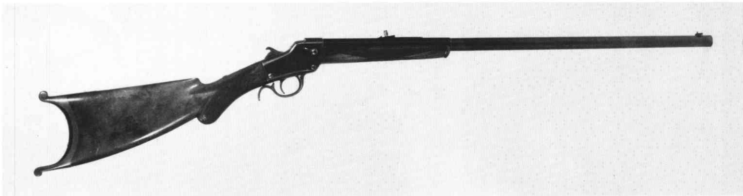
BAY STATE ARMS Co. "MATCH" rifle c. 1885-86 A single shot lever-action drop-breech target rifle manufactured by Willilam H. Davenport at Uxbridge, Massachusetts. This "match grade" rifle, serial no. 1067, has a checkered walnut stock and forearm, an iron "Swiss style" buttplate, and 28 inch half-round barrel in .32-40 cal.
