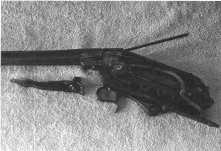
All at rest. The bottom of the swivel breechblock can be seen above and to the right of its lever.
