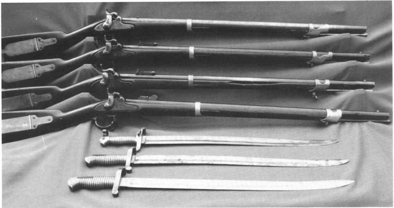
Top, an original M1841 dated 1846, then Benton/Snell altered 1841 rifle, .54 calibre; Benton/Snell bayonet altered 1841 rifle dated 1851/55, .54 calibre, and an 1854 dated Type II slide sight alteration of 1841 rifle, .54 calibre, with bayonets.
