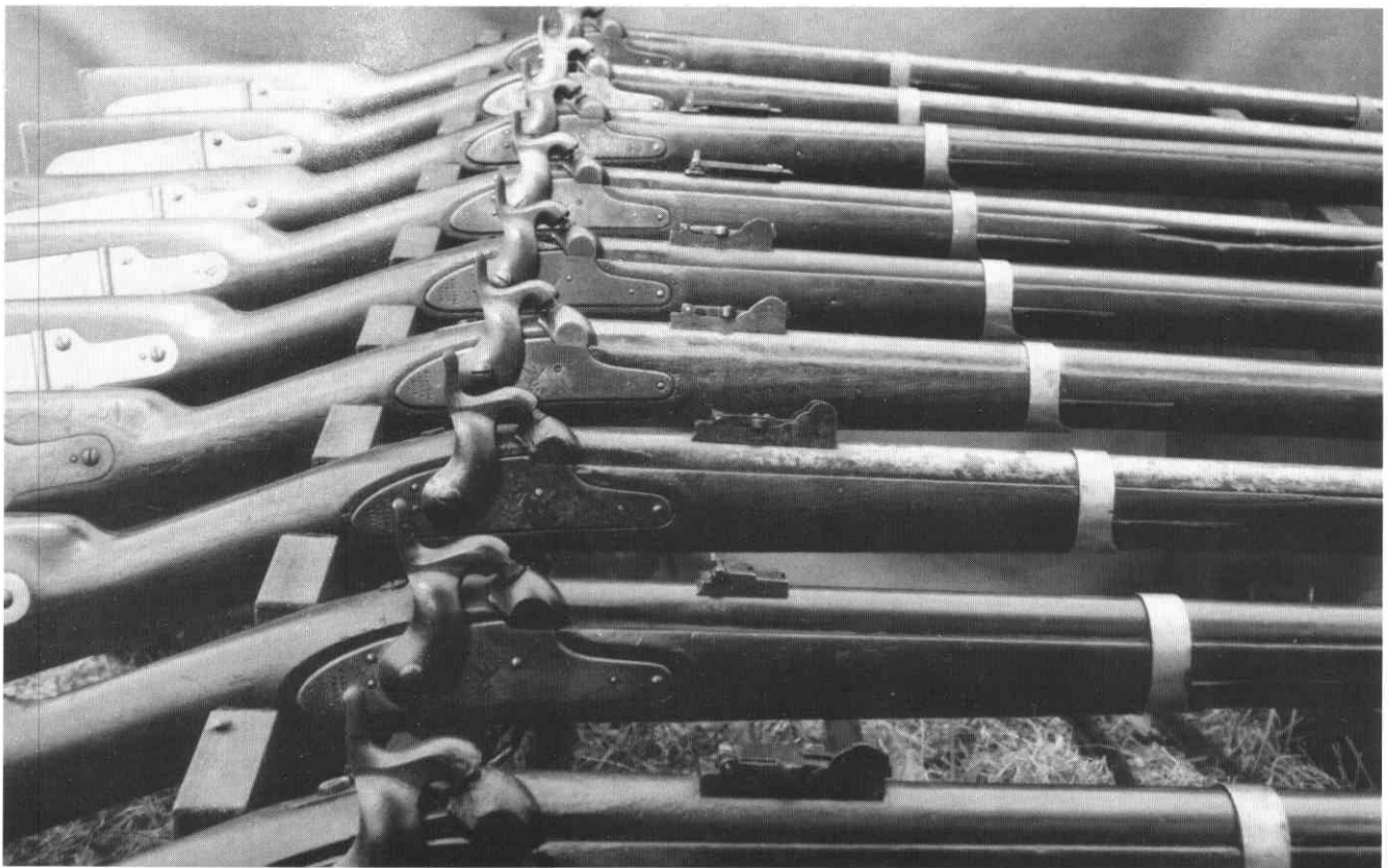
Composite shot of rear sight evolution. top, 1845 dated 1841 Whitney rifle, original sight. 2, 1846 dated Harpers Ferry 1841 rifle, original sight. 3, Benton/Snell screw sight. 4, Benton sighted, sword bayonet altered 1851/1855 dated. 5, Type II rear sight on 1854 dated 1841 altered from Benton sight. 6, Type II 1851 dated 1841, slide rear sight. 7, Type III slide rear sight, 1855 rifle sight. 8, Type IV 1858 rear sight. 9, Type III alteration on 1855 dated Whitney 1841 rifle.
