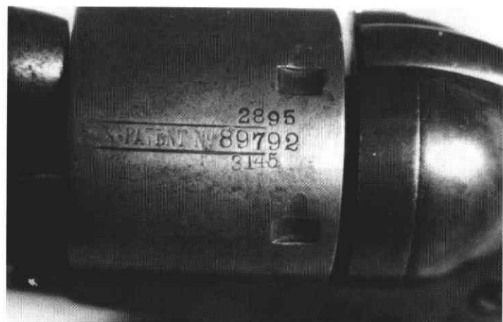
Figure 17: This cylinder has worked in at least two '61s besides its original '51, serial number 89,792. Cylinders are interchangeable and after alterations were renumbered to match the revolver, sometimes under the original number and other times on the rear face between the cartridge chambers. Serial numbers were left intact and old ones were not crossed off.
