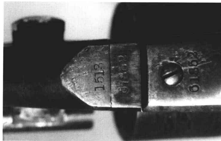
Figure 15: A '61 barrel very well adapted to a '51. These are found with no numbers or with numbers matched to the revolver placed above its original number. In the photo above the original barrel number was left intact and unenhanced.
