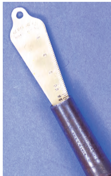
Figure 10. Caliber gauge inserted into cane muzzle.
