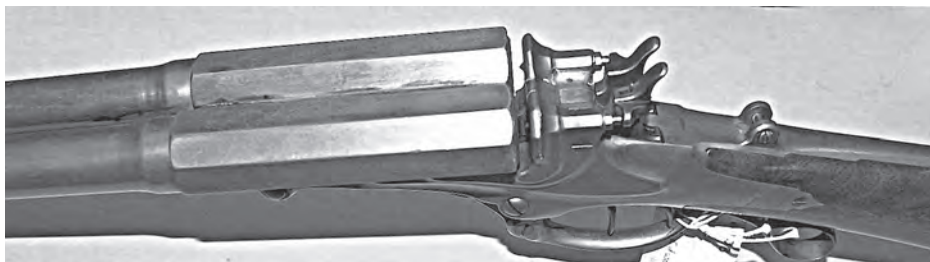
Figure 22. The action of Maynard's double rifle.
