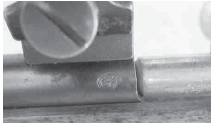
Figure 19. Model 67/677 proof mark relocated to clear scope base.
