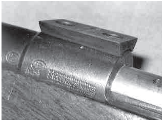
Figure 17. Low base used on rifles without metallic sights (Model 697 rear base shown).
