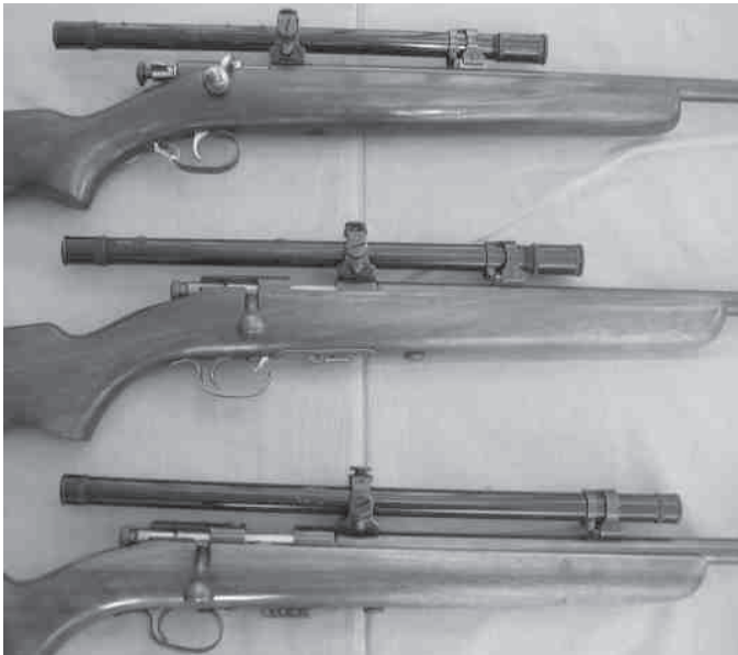
Figure 7. Close-up of the Model 677, early Model 697, and late Model 697. Note the different location of the rear scope bases on the early and late Model 697s and that the scopes differ in construction. The scopes are close to the barrels as see-through bases were not used. The top two scopes are 2 3/4-power and the bottom scope is 5-power.
