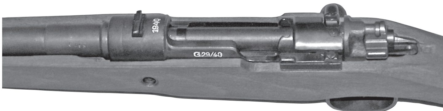
Figure 6. Steyr was one of the major producers of Volksturm rifles. Normally these are marked "Mod 98 bnz 45" on the receivers, but Steyr also used older receivers apparently from old part stocks like this 1940 manufactured receiver.
