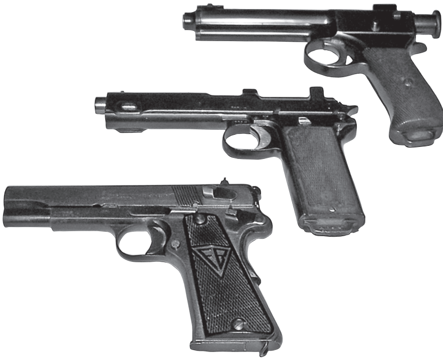
Figure 1. Steyr never excelled in pistol manufacture but was best known for rifle production both military and civilian. These three designs are the most often encountered handguns produced by Steyr: the Roth Steyr; the Steyr Hahn; and the P35 (P), produced under Steyr supervision at Radom Poland.
