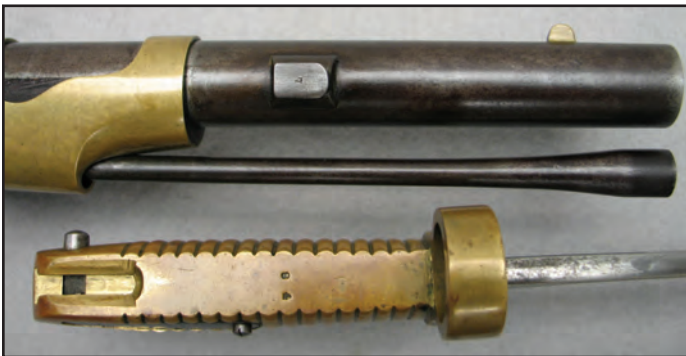
Figure 14. The New York Remington alteration used a stud brazed to the barrel and applied mating numbers to the stud and Collins bayonet.
