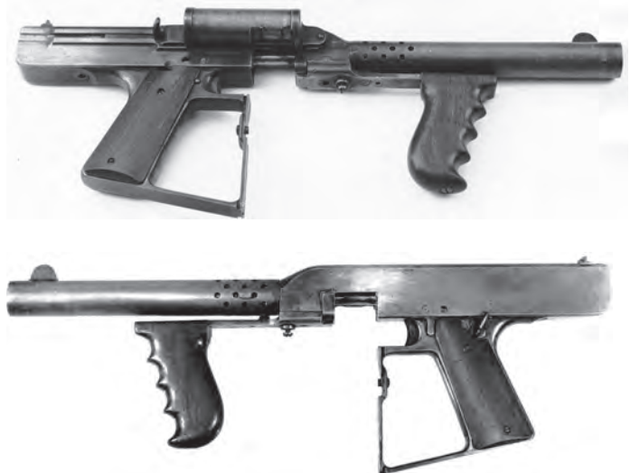
Figures 9. The “Persuader” Thompson Submachine Gun was the first version of the Model of 1919. This is a belt feed hand held firearm. The rate of fire was so fast that the web belt of ammo would jam the feed mechanism. (Photo credit West Point Military Museum)
