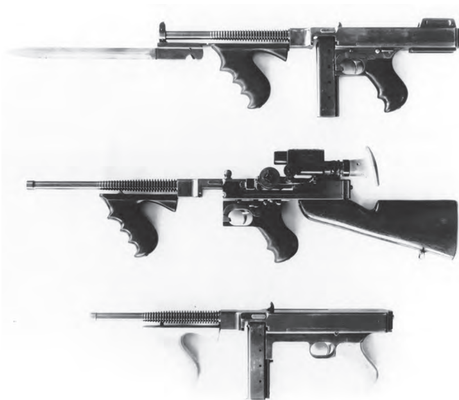
Figure 14. Early experiments with the Model of 1919 families included (left to right) serial number 3 with a bayonet attachment, another Model of 1919 with Warner Swasey sniper scope attached, and serial number eight.
