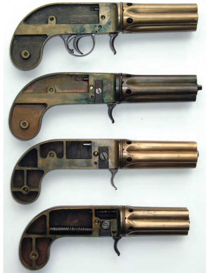
Figure 9. Budding pepperboxes with their right grips removed. From the bottom: Model 1; Model 2a; Model 2b; Model 3b. Note the simpler, open internal structure of Model 1, and the surprisingly long (and substantial) striker and its surrounding coiled spring. At the top of each is the short rod and spring for the barrel indexing system (see Figure 2). (Collection / Photo by Jas van Driel)
