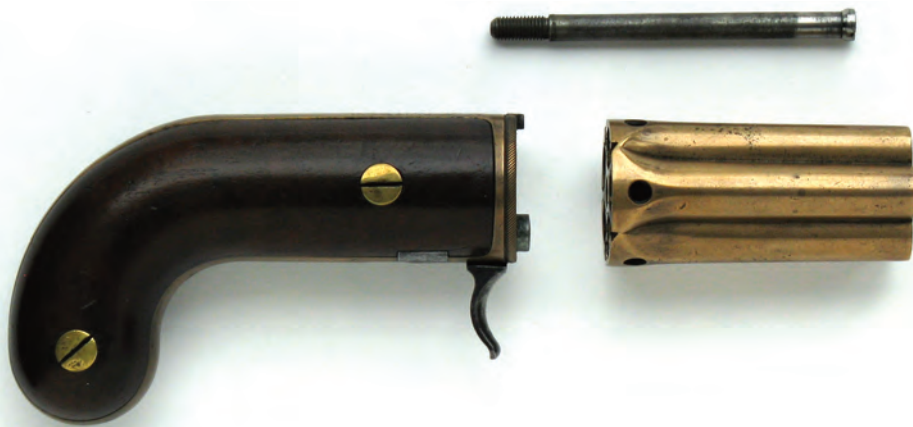
Figure 4. The barrel group retaining rod, and the barrel group, both removed. This is a Model 1 pistol, but the Model 2a removable rod would look the same. Note the head of the striker in the fired position. (Collection / Photo by Jas van Driel)
