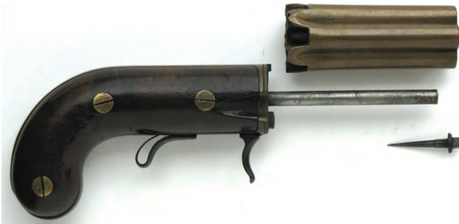
Figure 6. The barrel group removed from the frame-attached retaining rod, with the square-headed nut and pricker. This is a Model 3a pistol (with external capping slots), but the Model 2b would look the same. (Collection / Photo by Jas van Driel)
