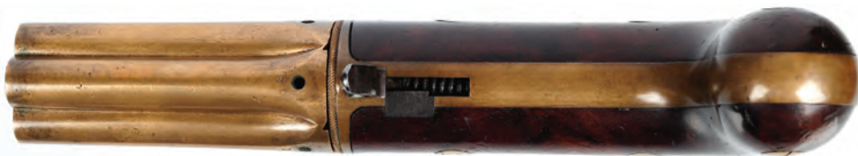
Figure 3. The spring-enclosed and -driven striker with integral cocking lever. Note the steel plate with small notch for holding the striker mechanism cocked. (Photo by Dan Retting)
