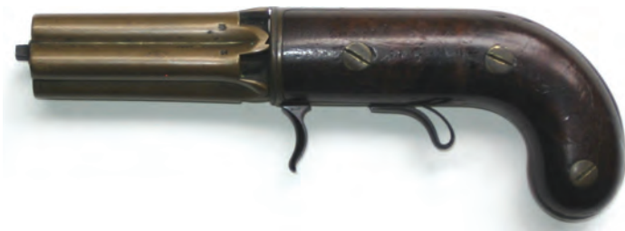
Figure 7. The only known Model 3a pistol, with external capping slots. Note the protruding square-headed nut at the front. (Collection / Photo by Jas van Driel)
