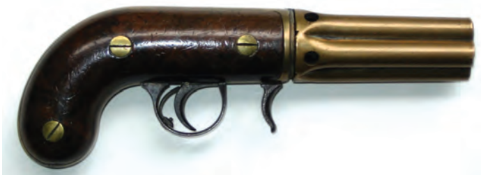
Figure 8. A Model 3b pistol. The barrel group attachment is not original, hence no square-headed nut is visible. (Collection / Photo by Jas van Driel)
