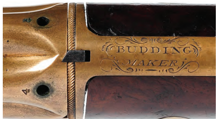
Figure 2. The steel catch (spring controlled) and tiny notches for indexing the barrels, and a typical "Budding Maker" marking on the top frame strap. Note also the vents and the barrel number. (Photo by Dan Retting)
