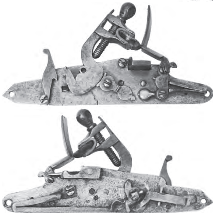
Figure 8. A classic Type 1 English lock c.1620, with a dog or back-catch for safety and buffer to arrest the forward movement of the cock. James D. Forman collection.
