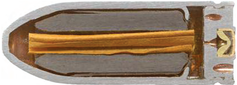
Figure 4. Sectioned Gyrojet showing the internal construction features. Actual size of the rocket is 13 mm or .51 caliber in diameter.
