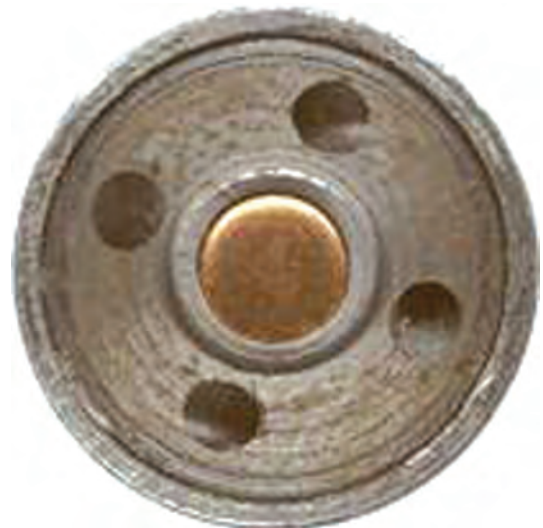
Figure 5. Gyrojet base showing primer in the center and the canted nozzles or ports that cause the rocket to spin in flight.
