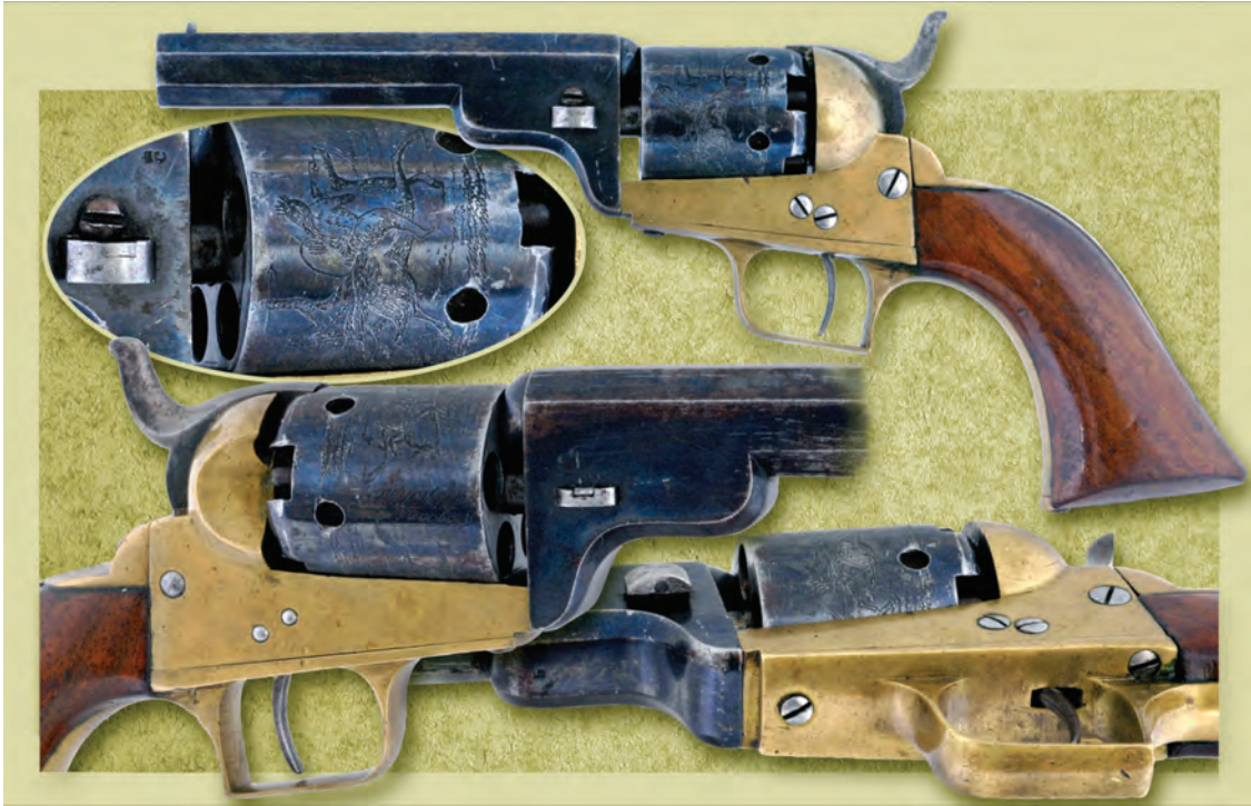
Figure 11. Colt Brevete "Baby Dragon" revolver with brass frame (Henry Stewart Collection, VMI Museum).
