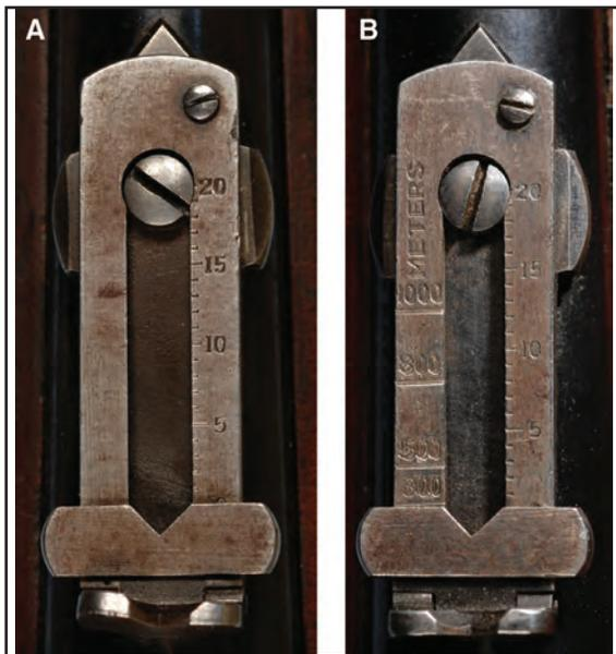
Figure 2. (A) Winchester standard Model 44A rear sight. (B) Modified sight found on the French carbines. When compared to the standard Winchester sight, it can be seen that the word METERS has been added to the left side as well as gradations from 200 to 1000.
