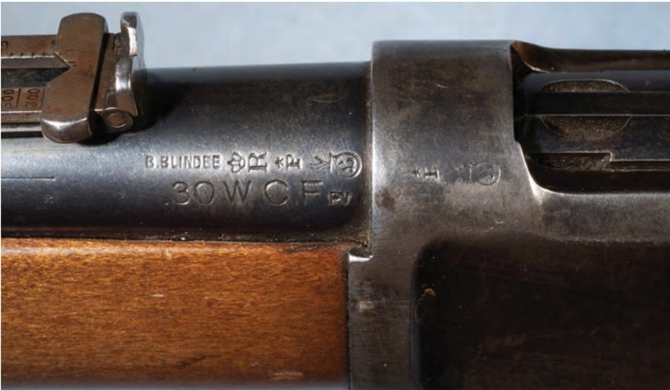
Figure 6. The Belgian marks on a Winchester.
