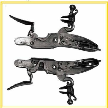
Fig 3. Lock internals: top, right lock with shallow pan for top barrel; left lock with deep pan for lower barrel.
