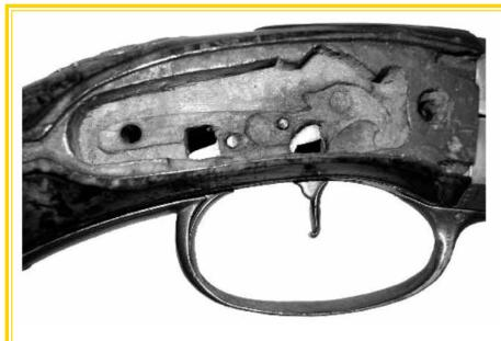
Fig 4. Stock cut out for right lock. Forward trigger serves top barrel by pushing down on sear of right lock while rear trigger pushes up on sear of left lock to fire lower barrel.
