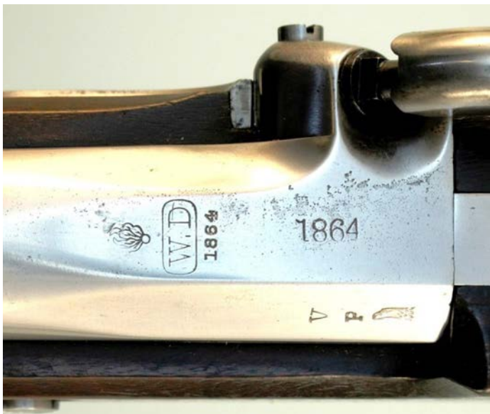
Figure 3. These marks are stamped into the barrel when a contractor's sample arm was accepted by the Ordnance Department as a "Standard Arm." A letter from the inspector to the contractor always accompanied the Standard Arm documenting the deviations from the Model Arm.
