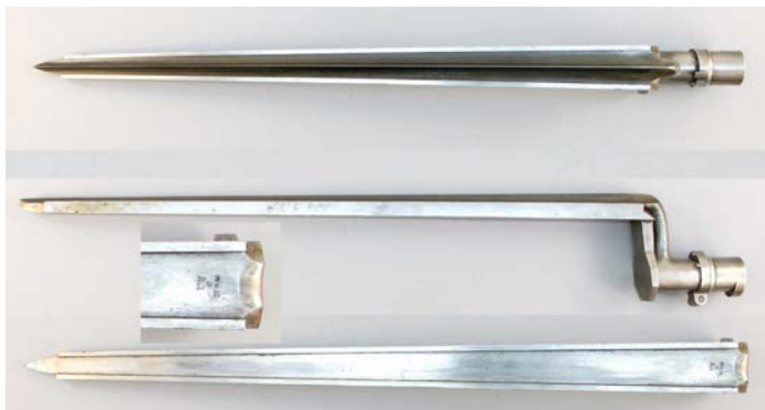
Figure 5. A verifying gauge, numbered "No. 46", is described as a "Receiving gauge for bayonets." There were only four verifying sets made, and five different bayonet gauges in each set. This gauge was part of the third set ("C") made in 1838. This gauge checks the dimensions of the blade and shank.
