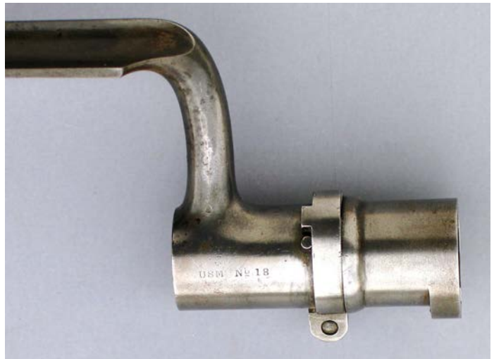
Figure 2. Pictured here is one of 24 Model Arm bayonets made by Harpers Ferry Armory in 1838. The socket of this Model 1835 bayonet is marked, "USM No. 18." The clasp stud and screw head are marked with an "M" stamp. This bayonet served as a model for the workmen to copy when they set up the tools and jigs in the armory.
