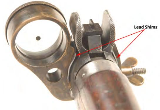
Figure 8 b. The offset Ulster/Neill objective with its prominent 4 MOA dot, a vestige from Bull's Eye shooting. Note the lead shims that were employed (today as in WWI) to stabilize the clamping of the sight in the muzzle cap's lightening grooves. (Author)
