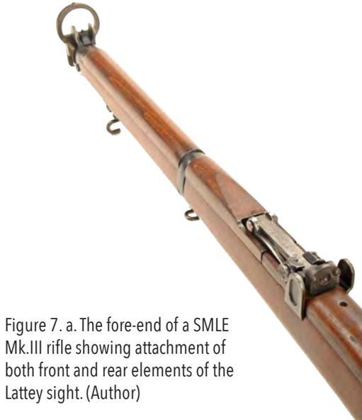
Figure 7. a. The fore-end of a SMLE Mk.III rifle showing attachment of both front and rear elements of the Lattey sight. (Author)
