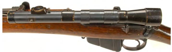
Figure 6 - Receiver area of an SMLE Mk.III fitted with a Periscopic Prism Co. telescopic sight. The magnification of this sight was the same as that of the Galilean sights, and both were in service in 1915. (Author)
