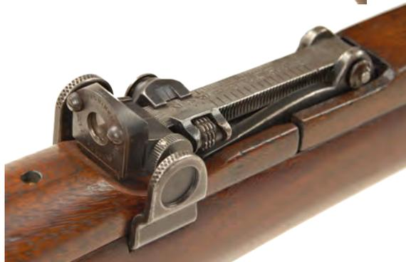
Figure 7. b. Close-up of the Lattey's ocular lens holder attached the standing leaf of an SMLE Mk.III. The radius of the handguard behind the sight needed to be relieved slightly to allow full depression of the elevator, otherwise its graduations are useless. (Author)
