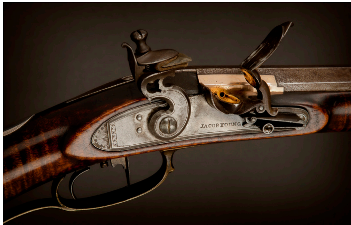
Figure 2. Jacob Young produced this exquisite handmade lock at a time that English flintlocks would have been readily available. Its waterproof flashpan and inset frizzen cover is lined with pure gold. Note the gold flash guard dovetailed into the barrel surrounding a gold touch hole liner.
